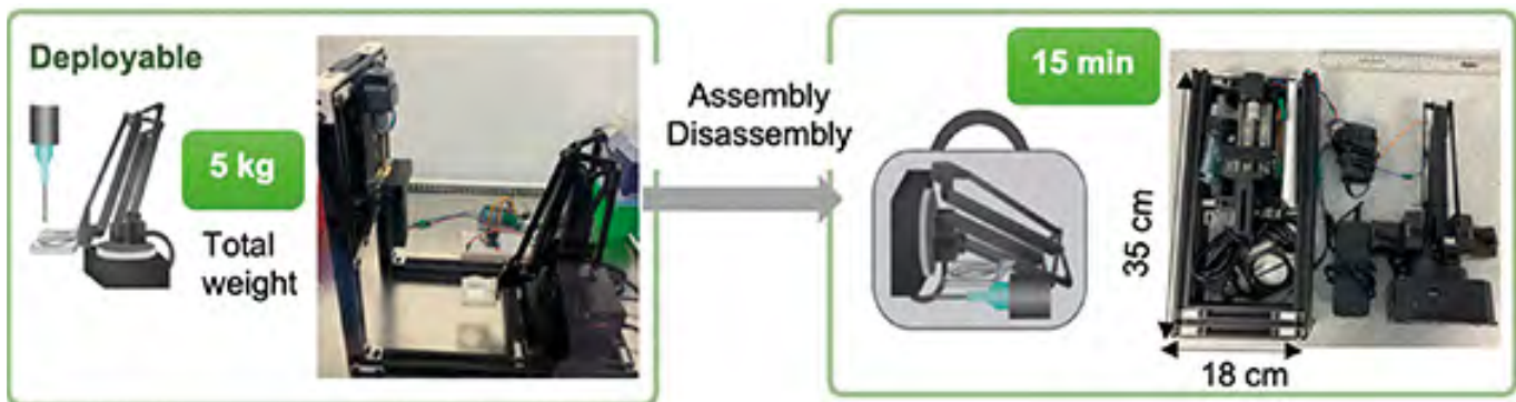
The deployable printer can be folded, transported, and easily re-assembled. © 2023, Mazzaglia et al., licensed under CC-BY 4.0. Reproduced from Biofabrication 15, 025005, https://doi.org/10.1088/1758-5090/acb1db .
