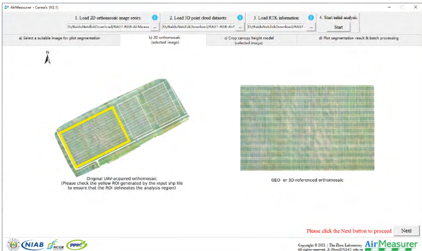
Graphic user interface (GUI) of AirMeasurer when batch processing a series of 2D orthomosaics and 3D point clouds for 2D/3D trait analysis of thousands of 12-m yield plots at the RAGT field trial in the UK. © 2023, The Zhou Laboratory, licensed under CC-BY 4.0 (individual, open license).
